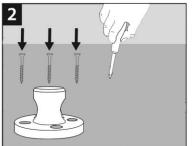
Use the screws provided in the pack to secure the GX-1 to the floor
