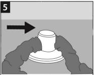
Pull the flex chain through the hole and get it into position
