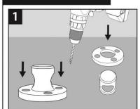
Place body into the position then place base plate over the body and drill holes accordingly
