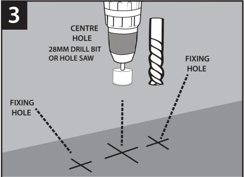
DRILL CENTRAL HOLE WITH A 28MM DRILL BIT OR HOLE SAW DEPENDING ON SURFACE. THEN DRILL FIXING HOLES 3MM DRILL BIT FOR WOOD /10MM FOR CONCRETE OR CERAMIC
